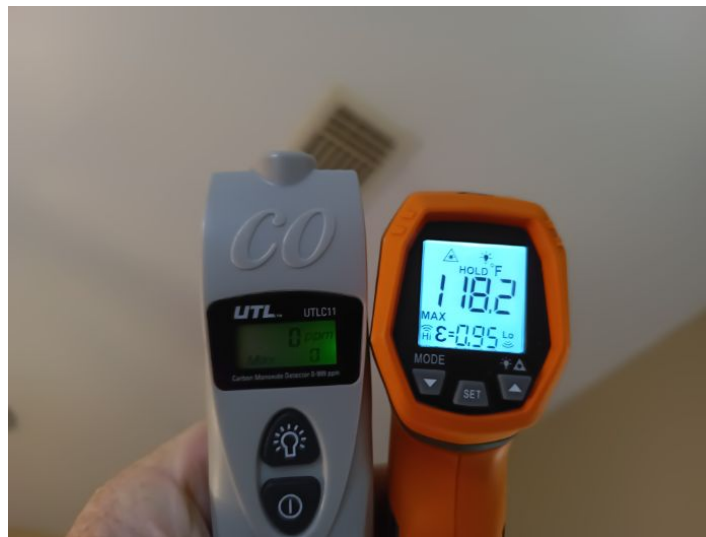
118.2 degree heat, 0 ppm carbon monoxide
