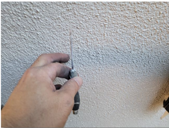
5- 1.3 Test Location F - Soft substrate encountered
