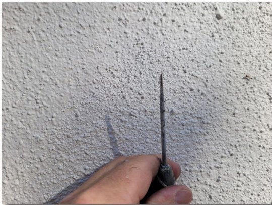
2- 1.3 Test Location C - Soft substrate encountered
