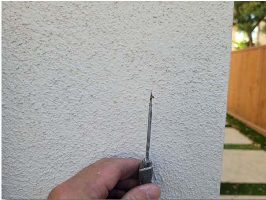
1- 1.3 Test Location K - Soft substrate encountered
