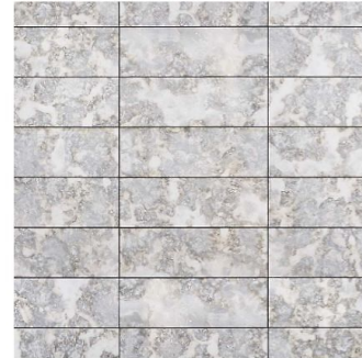
BACKSPLASH SOHO STUDIO, OLD WORLD SERIES MRROLDWRLDAR6X18 8X18 STRAIGHT STACKED HORIZONTAL (MIRROR CAULKING- NO GROUT)
