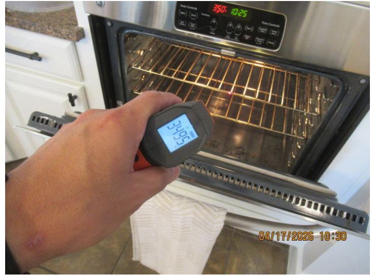
Oven temperature was within acceptable range. Acceptable range is + or - 25 degrees when oven is set at 350 degrees.
