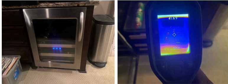
Units 1 Wine Fridge Only: Thermal Temperature readings, Photo of cool temperature
