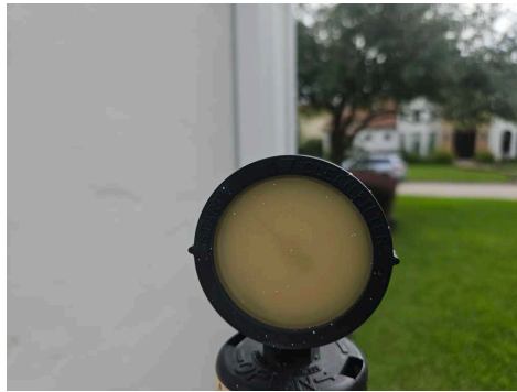
Filter gauge cloudy / damaged
