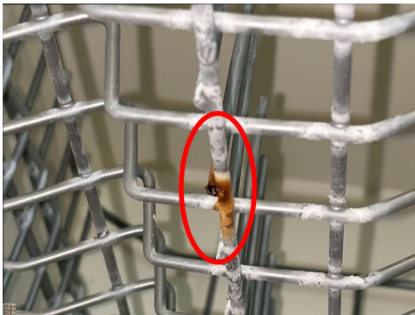
Rust on trays
