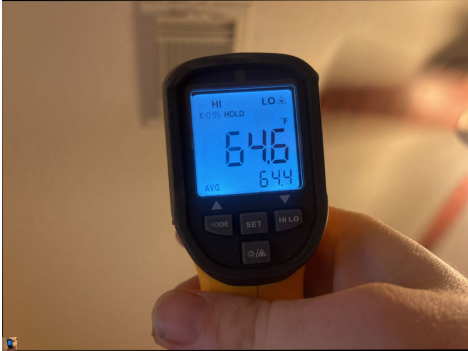
Bedroom 1 vent temperature
