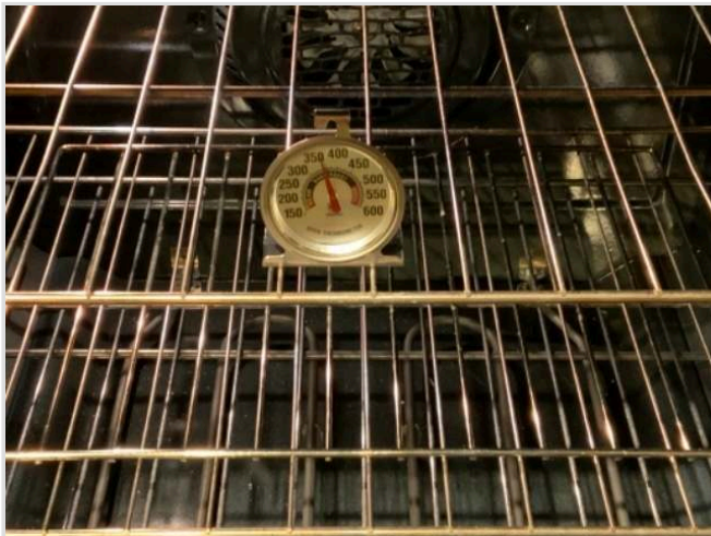
Oven temperature reading (approximately 360 degrees - within tolerance)
