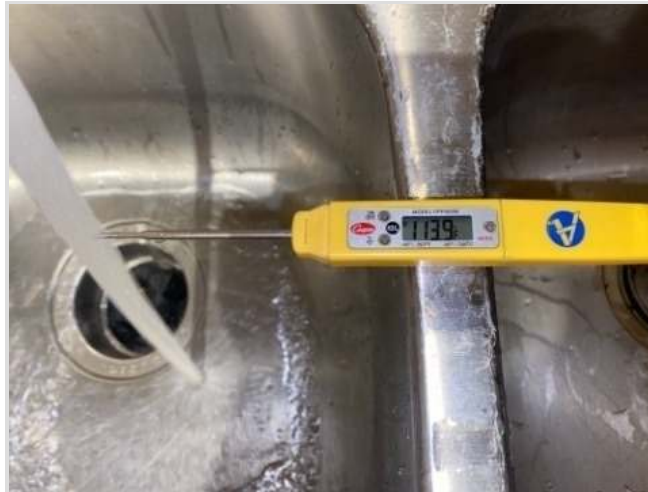
Measured hot water temperature (kitchen sink): 113.9 degrees
